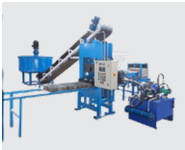
Flyash Brick Plant
